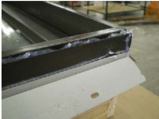
Figure 18. Section Detail of Sealant Location
