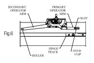
Twist the head of the screwdriver and pop the arm from the stud. If you push or pull the lock side of the sash, it will swing slightly back and forth. On the inside face of the sash is an operator track. The top of the track has a note specifying "DEPRESS ARM TO DETACH" and an arrow. Located at the end of the secondary arm is a roller.
