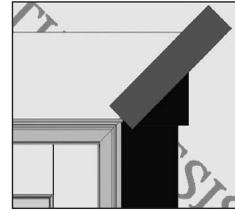
*Note: Rigid flashing must run at least 1/8" past the brickmould.*
