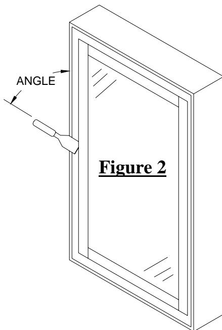
The brackets are 1" wide with holes in both ends to attach the sash to the frame. These brackets are hidden behind the side stops on stationary units and picture units with glass widths less than 38", or on all four sides on picture units with glass widths on or over 38". In order to remove sash the wood inside stops must be removed to expose brackets.
