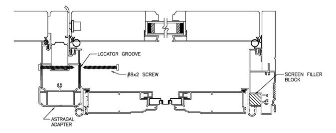
Step 4: Install the swinging screen per the instructions provided with the screen system.
