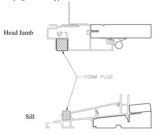
Step 2: Set the base (angled cut end) of the screen adapter over the sill foam plugs while engaging the back of adapter with the face of the astragal. Make sure the top of the adapter clears the frame at the head of the door unit and push inward until it bottoms out.
