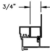
CLAD BRICKMOULD CASING
